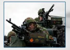
The ISTEC Mk1 UGM undergoes trials on the WMIK Land Rover. It was designed to offer a stable firing platform for the 20mm GIAT cannon and 12.7mm HMG.
